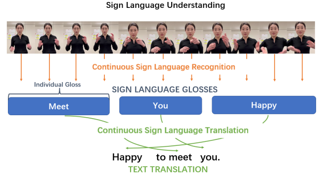
Fig. 1. Sign Language Understanding pipeline. The Sign Language Understanding system conducts CSLR task as the first step to tokenize the input video into glosses. The next step is to translate the glosses into the corresponding spoken language text.
